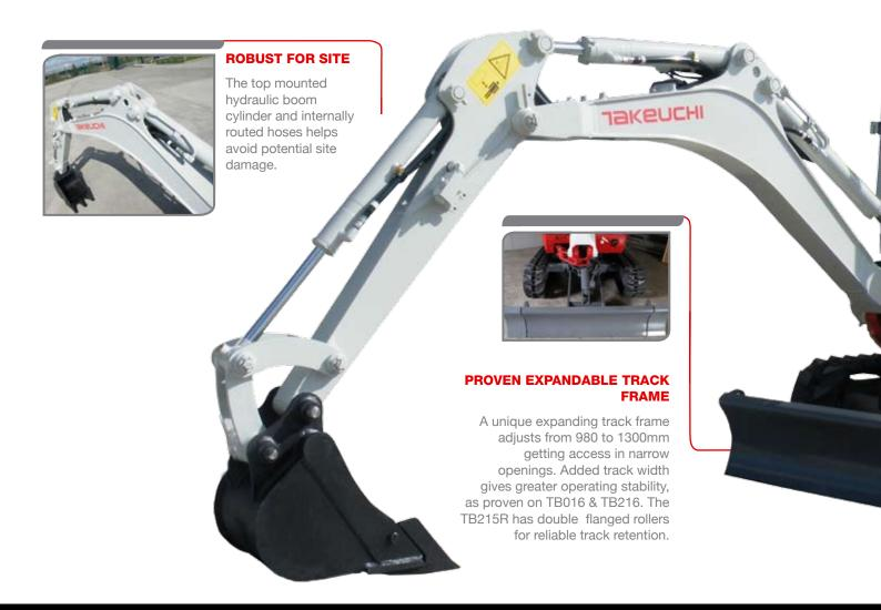
The TB215R is a very well protected mini digger built for the toughest site conditions.
