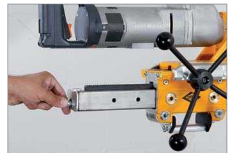
mounting a securing sheet against unintentional removal of the carriage
