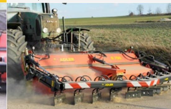
Combination scraper/sweeping machine K 750 with dirt collector
