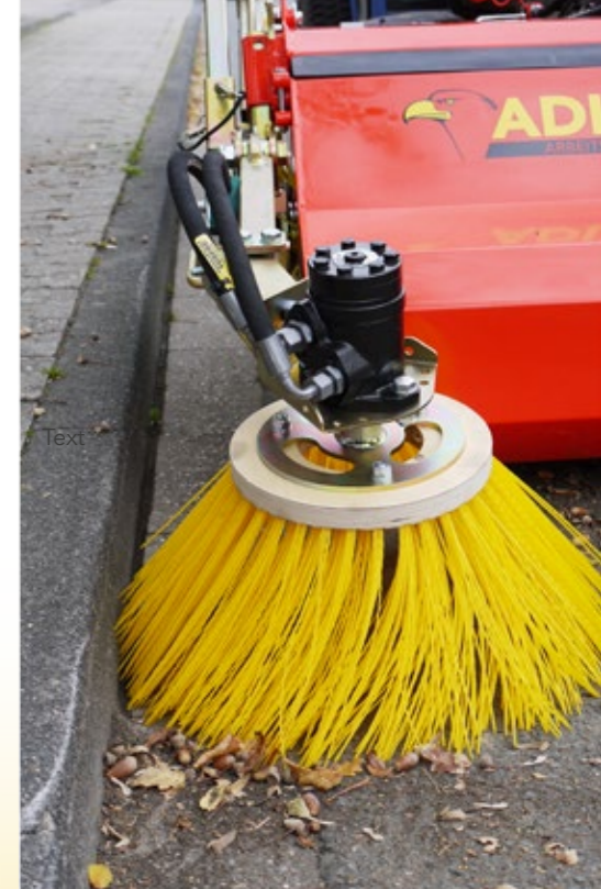
Rotary side brush in use
