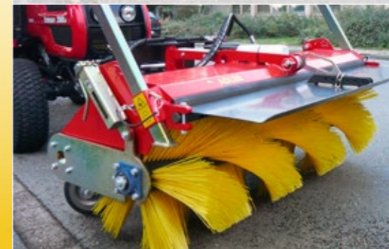
K 560 with adjustable splash guard
