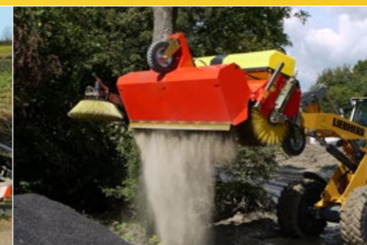
Hydraulic hopper emptying system
