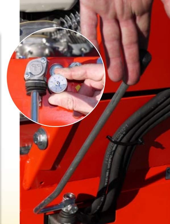
Hydraulic rod steering system and stepless traction drive
