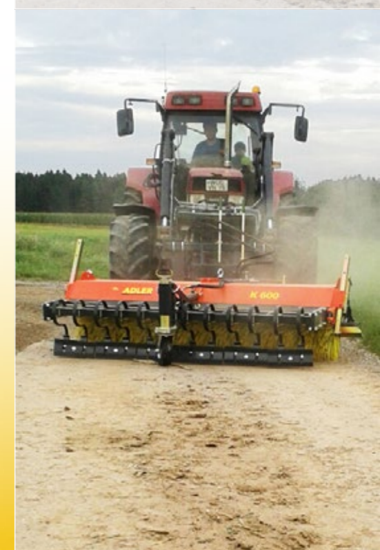
KV-series Scraper Attachment with third support wheel
