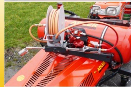
Available on option: Hand-held burner kit incl. 15 m-hose reel
