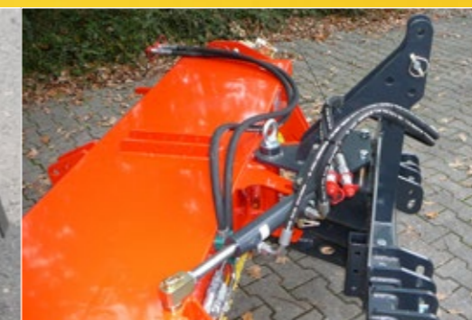
Three-point linkage, CAT I/II
