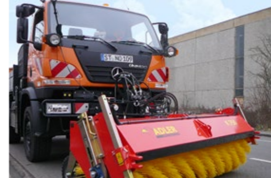
Unimog Attachment incl. lifting system acc. to DIN 76060
