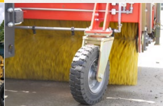
Three large wheels 400 mm x 100 mm
