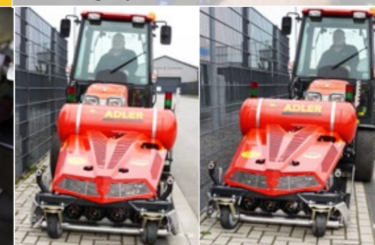
Hydraulic side shift 20 cm to the left and right
