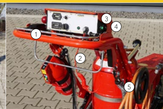
1) Backwards/forward drive 2) Safety cable to stop motor 3) Securing mount 4) On/off switch 5) Hose bracket
