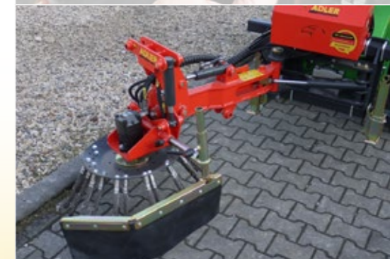
Heavy brush head with protective side guard
