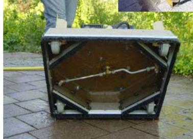
A rotation arm with 2 nozzles close to the surface effects the intensive cleaning
