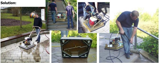
Easy-Clean EC 60 is cleaning surfaces and joints at a time, the jet of water is hold under a protection cover
