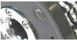
Drum with replacement bushes = longer service life
