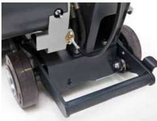
Foot lever for transport position = fast machine relocation
