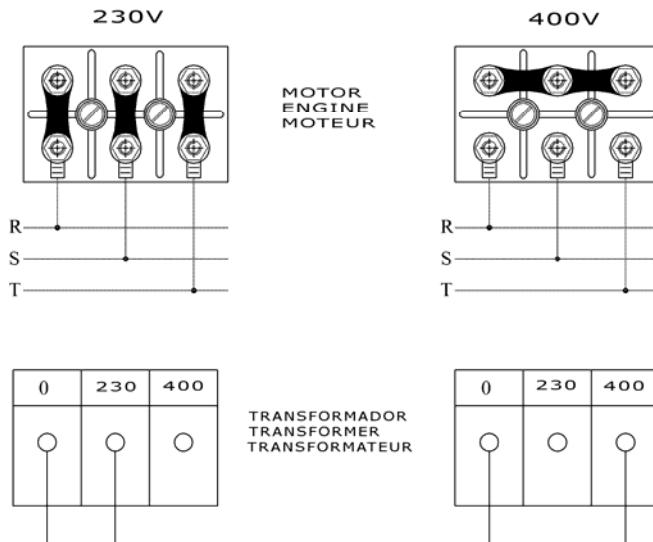
**IMPORTANT:** It is appropriate to change the position of the bridge plates in the engine terminals. It is also important to change the adhesive labels indicating the voltage, to reflect the change made. **It is very important to unplug the machine before changing the voltage.**
