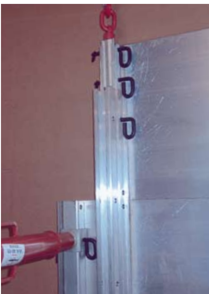
3-D lifting eye suitable for aluminium panel connector and LITEBOX strongrails
