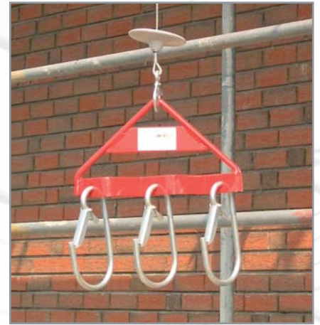
Hoisting chain for scaffold elements
